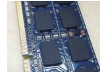
ICチップの封止材に用いられるシリカ粉 Silica Powder used as an EMC filler for IC chips
